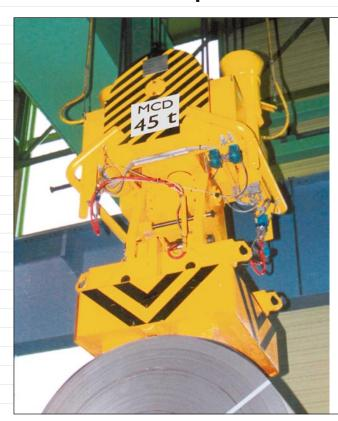
Hook block on automatic crane with slewing gear, lockable gimballed load suspension and calibratable weighing equipment
